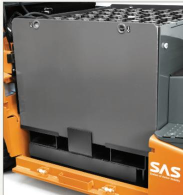
Battery mounted on optional rollerbed for easy extraction. Alternatively, fork pockets allow another forklift to remove the battery.
