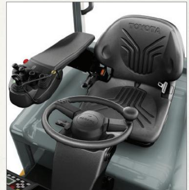
Fully adjustable Operator Restraint System (ORS) with side-wings and lumbar support.
