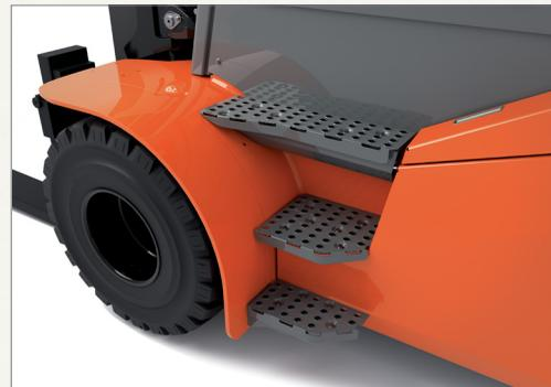
Large entry window with wide steps and double driver assist grips ensure fatigue is minimized in applications that require repeatedly getting in and out.
